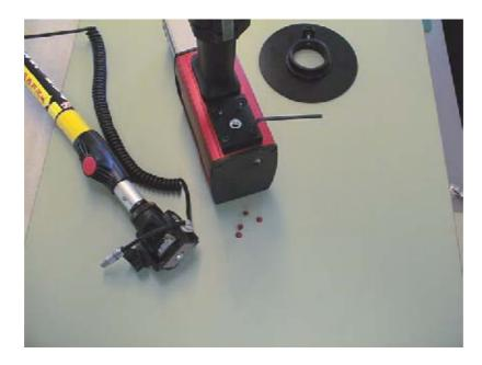
2. Mount the Adapter plate in the thread hole underneath the RetroSing. Use the 4 screws.
