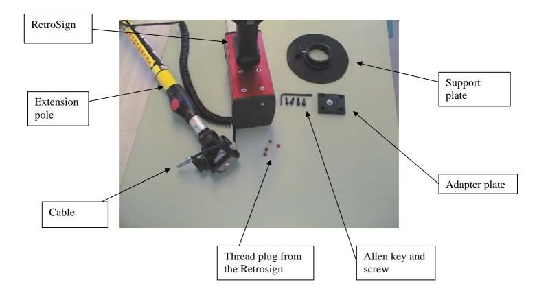
1. Remove the thread plug from the Retro Sign (red plugs underneath the RetroSign).
